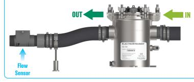
The "BEST" location for the ClearVis Flow Sensor is after the Canister output with at least 12" of straight hose before and after the Flow Sensor. The ClearVis Flow Sensor can also be installed on the pressure side of the pump.
