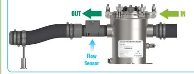
An "ACCEPTABLE" location for the ClearVis Flow Sensor is on the output of the ElectroStrainer Canister with at least 12" of straight hose after the Flow Sensor.
