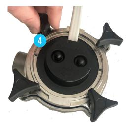
5. Remove the Electrode Assembly and pressure ring by lifting it straight up by the sides of the black plastic top. Do not lift or pull on the top cable connectors.
