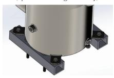
Mount canister on Base Tab Extension Brackets.
