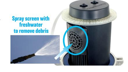
NOTICE Low seawater flow may damage cooling system and other components that depend on this water for proper operation. It is the owner's responsibility to monitor the vessel's seawater flow and perform any maintenance on the vessel's seawater pumps, strainers, and screen in ClearCell.
