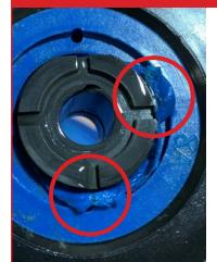
Lower-grade composites are more susceptible to overheating, premature wear, and failure due to friction.
