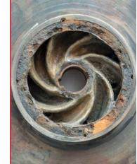
Metallic parts in the seawater fluid path are susceptible to corrosion, erosion, cavitation, and eventual failure.
