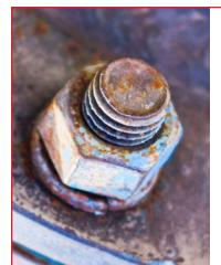
Other pumps use low-grade painted steel hardware that is not made for the marine environment.
