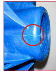
Unreinforced heads crack if excessive force is used or the threads are compromised.
