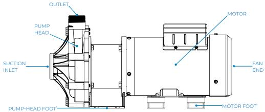
\*Pump-head foot and motor foot not included on all models
