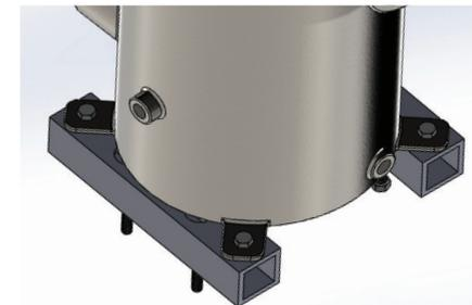
1. Mount canister on Base Tab Extension Brackets.
