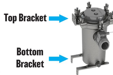
1. Attach Top and Bottom Side mount brackets to the canister with (4) M5 machine screws.
