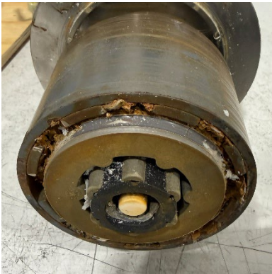
Motor damage due to running dry
