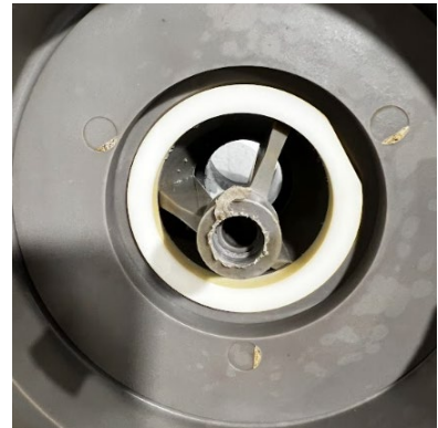
Pump face damage due to running dry
