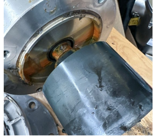
The presence of rust indicates a wet-end breach.
